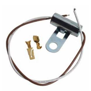
The white wire leads to the tach wire; the brown wire leads to the distributor connector. Bolt the filter casing to a suitable ground (i.e. intake manifold or nearby ground source).
