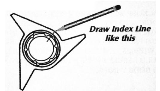
This will give you an immediate reference point to see if the Spinner is properly tightened during the test drives. After each Spinner/Adapter Assembly is indexed, lower the vehicle to the ground and drive the car slowly while listening for any "clicking" or other strange sounds that may indicate a Knockoff Wheel is not properly tightened. A Knockoff Wheel that is coming loose will also make the car wander from side to side and a lack of control will be evident.
