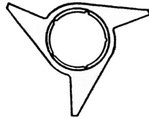
**Right Hand** — Wings point in a clockwise direction. Spinner tightens onto Adapter in a counter-clockwise direction.
