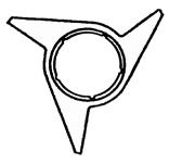
**Left Hand** — Wings point in a counter-clockwise direction. Spinner tightens onto Adapter in a clockwise direction.
