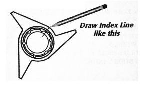
This will give you an immediate reference point to see if the Spinner is properly tightened during the test drives. After each Spinner/Adapter Assembly is indexed, lower the vehicle to the ground and drive the car slowly while listening for any "clicking" or other strange sounds that may indicate a Knockoff Wheel is not properly tightened. A Knockoff Wheel that is coming loose will also make the car wander from side to side and a lack of control will be evident.
