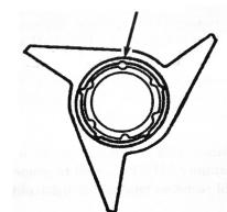
**Note**: The Anti-theft Pins are not designed or intended to prevent an improperly installed Knockoff Spinner from loosening and a Knockoff Wheel from coming off a car. The Anti-Theft Pins are intended to add an extra measure of security against theft by increasing the number of steps and time required to remove the wheels from the car. They are not a substitute for proper attention to detail during the installation process.
