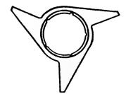
**Right Hand** — Wings point in a clockwise direction. Spinner tightens onto Adapter in a counter-clockwise direction.
