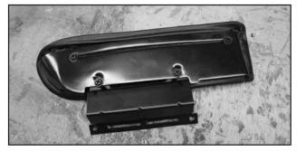
5. Place hinge in position over the alignment pins and fasten all four screws.
