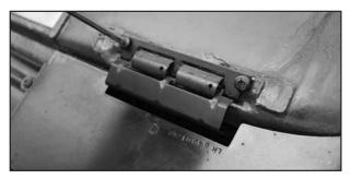
2. Place the old door panel face down and remove the two screws on back of the panel that secures the hinge to the panel.
