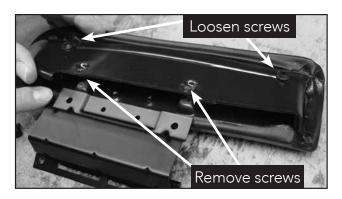
4. Remove the two screws from the new lid that will hold the hinge. Loosen the top two screws.
