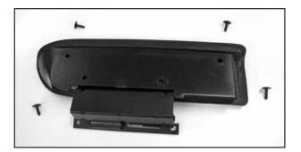
3. Remove the Compartment Lid from the old panel. Then remove the four screws from the underside of the compartment lid. Separate the hinge from the old Compartment lid.
