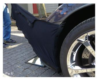
**Note:** Take extra-care when stretching the mask over and around the Splitter or Spoiler, rough edges and corners on groundfx can damage the mask over repeated installations.
