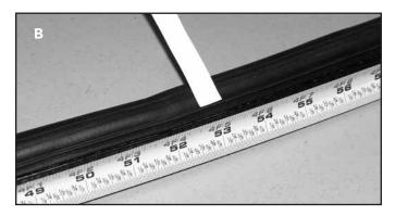
**B.** Measure the long side arc and mark the center with masking tape or a Post-it Note.
