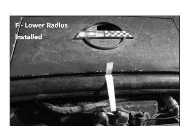
**F.** Next, start in the center of the back of the car installing new weatherstrip from the center to corner turns and press into place.
