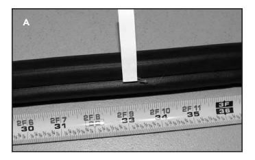
**A.** Measure the long straight edge and mark the center with masking tape or a Post-it Note.
