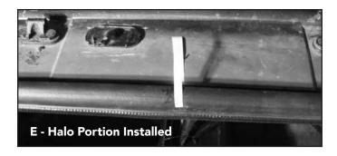
**E.** Index the center of the straight side of the weatherstrip with the top of the halo and press into place along the top edge to the point where the radius of the halo turns down on both sides. Do not do anything with the corners at this point.
