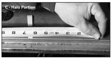
**C.** Halo Portion — Find the center of the halo portion of the car and mark that with the masking tape or Post-It note.
