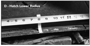
**D.** Hatch Lower Radius — Measure the center of the hatch lower radius and mark it with masking tape or a Post-It note.
