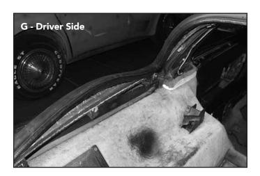
**G.** Work the excess of the weatherstrip into the driver's side corner pressing the excess from the curve parts into the corner.
