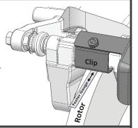
Caliper Cover should rest directly against the face of the brake caliper. The installer should verify that the bridges are set to 88°as depicted on image. Installer may adjust as needed.
