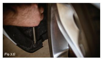
After removing the retaining pins, install a J-clip (Nipple side is toward the front of the car) at each of the two holes in the bumper. [The J-clip is designed to go around the edge of the fiberglass bumper or inner liner and serves as the nut for the screw you will be installing. Reposition the fender liner aligning the holes in the liner with the holes in the bumper. Now install the two (2) snap-head screw studs. Repeat this step on the other side of the car.
