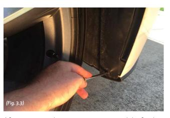
After removing the retaining pins, spread the fender liner to gain access to the bumper and install a J-clip (Nipple side is toward the front of the car) at each of the three holes in the bumper.
