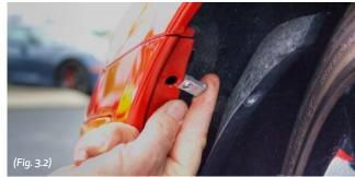
**Note:** the pin is a male/female assembly. The male piece can be pried loose from the female piece using a flat blade screwdriver. Insert the blade of the screwdriver in the slot at the edge of the pin and twist the screwdriver causing the pin to come free of the female piece. After removing the male piece, the female piece can be easily removed.
