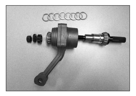
**4.** Assemble the spindle outer bearing tubular spacer and a .145" shim over the setup tool next to the tubular spacer.
