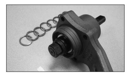
**5.** Place the tool into the spindle support & install the inner bearing, black spacer, large washer & nut.
