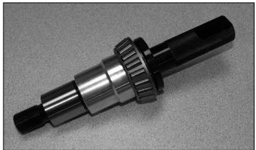
**3.** Place the tubular spacer with the large end against the outer bearing.
