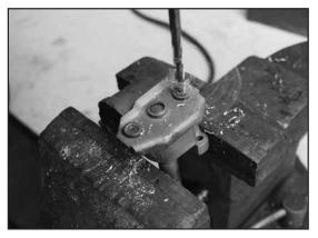
Step 1 With regulator assembly secured in vise. Drill the peened over rivet heads with a 7/32" drill bit.
