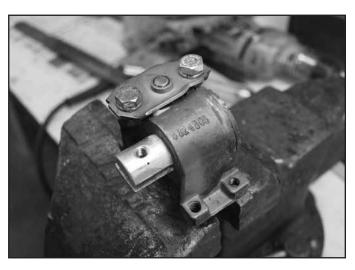
**Step 11** — Install  $1/4" \times 20 \ 1/2"$  bolts & lock washers to complete assembly.
