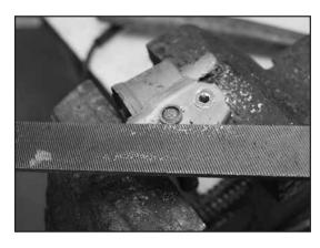
**Step 2** — File rivet heads flush to retaining bracket.
