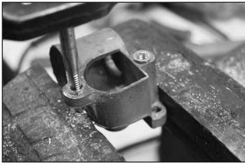
**Step 7** — Using a 1/4" x 20 Tap thread holes for assembly.
