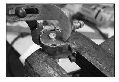
**Step 10** — Install end cap & fold over housing lip with channel lock pliers. This will retain the cap & gear assembly.
