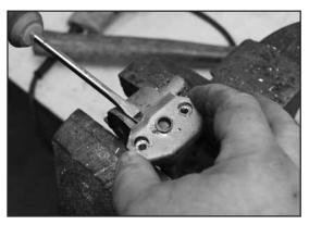
**Step 3**Pry off retaining bracket.
