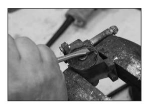
**Step 4** — Tap back folded over housing lip to remove end cap.
