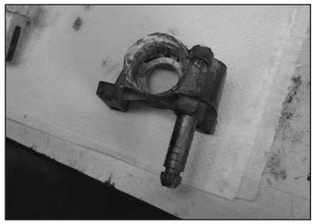
**Step 9** — Install the C-ring, then regulator shaft.
