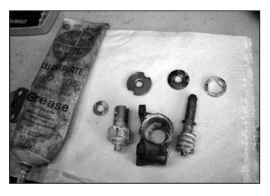
**Step 8** — Grease gears & housing with white lithium grease.
